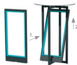
folding-system of the SET Table
