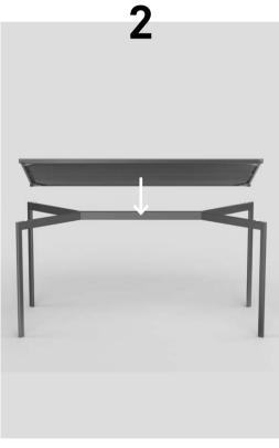
Lift top onto legs – make sure that the locator plates sit on the pins
